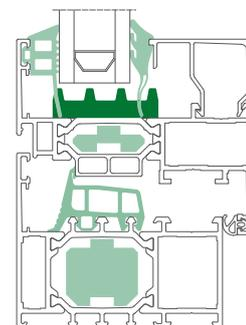
Super High Insulated:  $U_f = 1,53 \text{ W/m}^2\text{K}$
